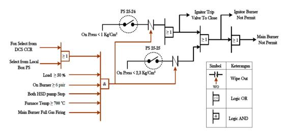
Figure 1. Modified logic diagram at DCS CCR
